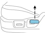
Before returning the seatback to its original position, make sure that cargo or any objects are not trapped behind the seatback. After returning the seatback to its original position, pull on the seatback to ensure that it has fully latched. An unlatched seat may become dangerous in the event of a sudden stop or collision.
